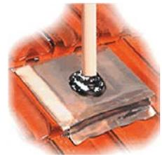
Best draw performance is obtained using a straight flue; this often means using a Tile Flashing. One example, shown on the right, is malleable and soft enough to be moulded over tiles. Another example is a Boot Flashing for use especially on corrugated metal roofs. This second example also has a high temperature variant for use within 2 metres of the Stove outlet.
