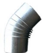
If the flue run is unable to go straight up and it has to come out of the wall, use two 45° bends (right) with a short straight length between them to allow for the wall thickness. Continue the flue run vertically up as far up as possible.
